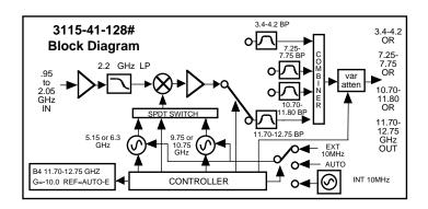
FIGURE 1.2 3115-41-128# Block Diagram
