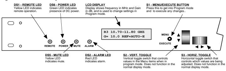
FIGURE 2.2 3115-41-128# Front Panel Controls and Indicators
